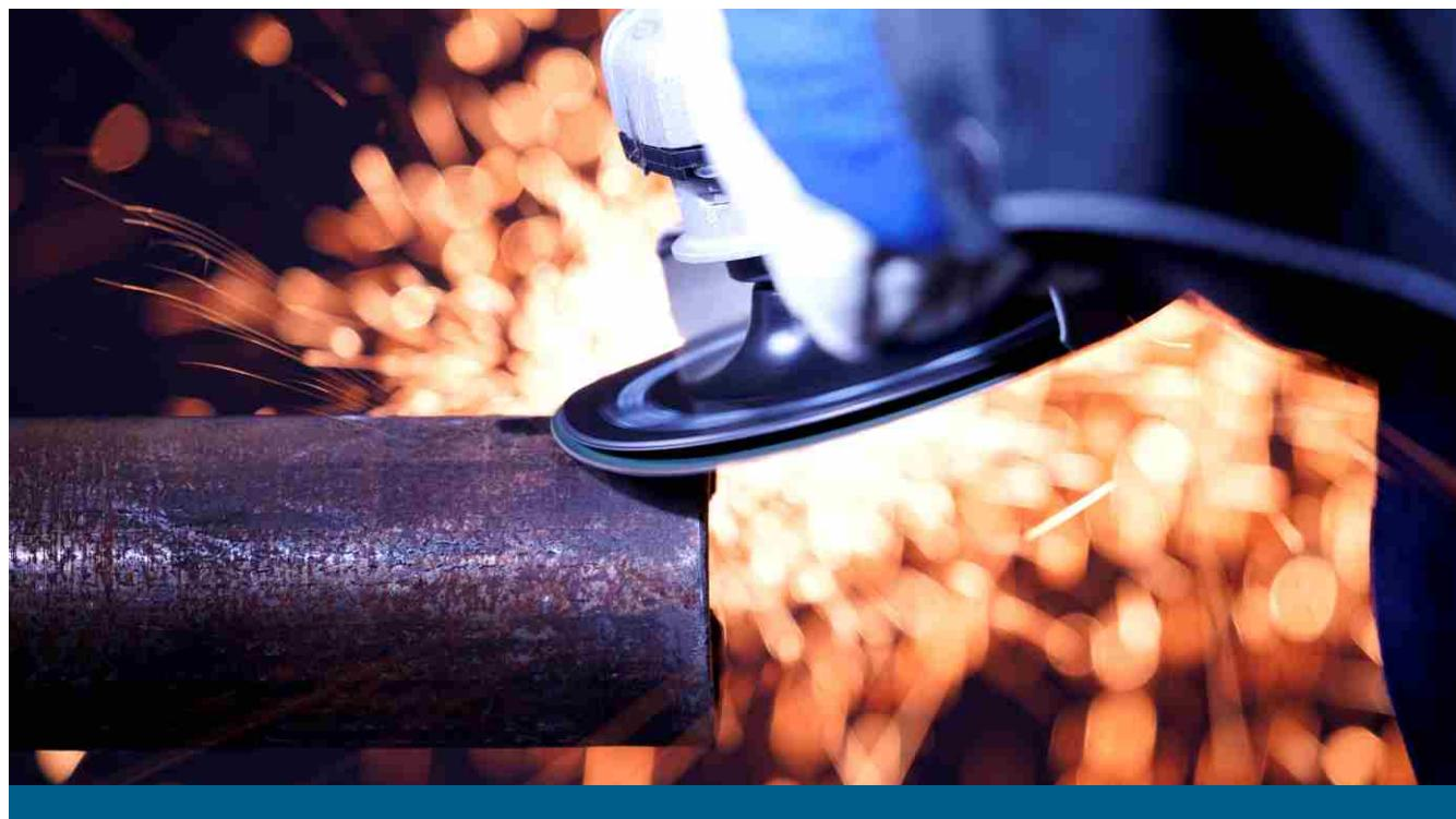
The 931 Fiber **100%** Zirconia line of fibre discs achieves exceptional levels of performance in metal grinding. The Zirconia Alumina grains provide very fast cutting rates and exceptional lifespan.
